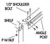
Insert shoulder bolt thru post hole and shelf hole (Fig.1). Connect 4 point lock nut (Fig.2) and tighten shoulder bolt (Fig.3). When all connections are completely tightened, this unit forms a rigid structure.
